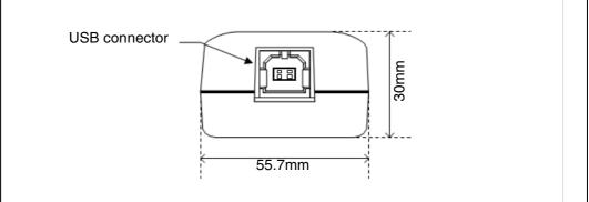
Figure 2 Adapter appearance (front view)
