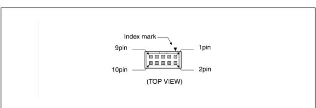
Figure 7 Adapter interface connector pin configuration
